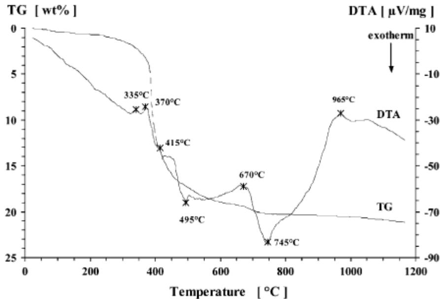
Figure 2: DTA-TG analysis of commercial colemanite. [11]
