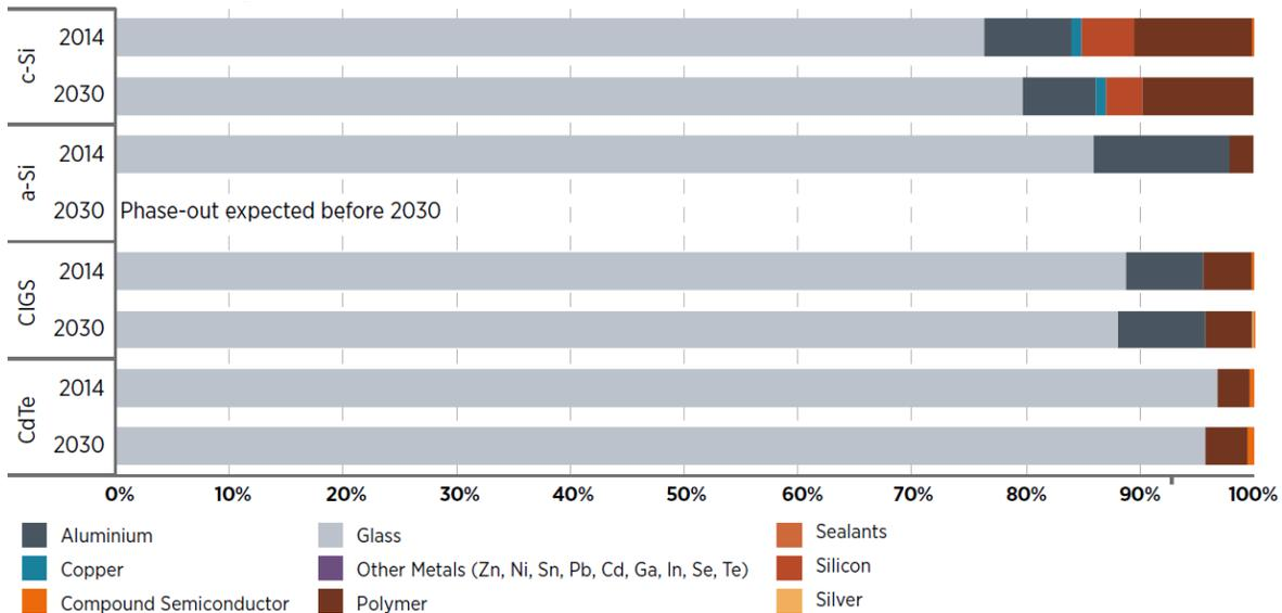
Figure 3: Evolution to 2030 of materials used from different PV panels technologies as a percentage of total panel mass. [46]
